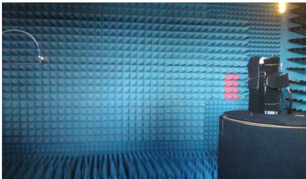
Measurement of antenna radiation characteristics in LHFT anechoic chamber
